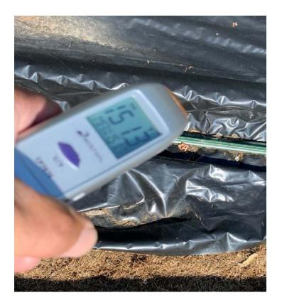
This surface temperature of 151.3 Degrees was on a partly cloudy 74 Degree day. But what really counts with Soil Solarization is the temperature below the surface where the weed seeds, nematodes, bacteria and fungus reside. A few spot checks showed that on this same day temperatures 4 inches deep were an astonishing 147.9 Degrees. Soil Solarization definitely can work in Minnesota!
